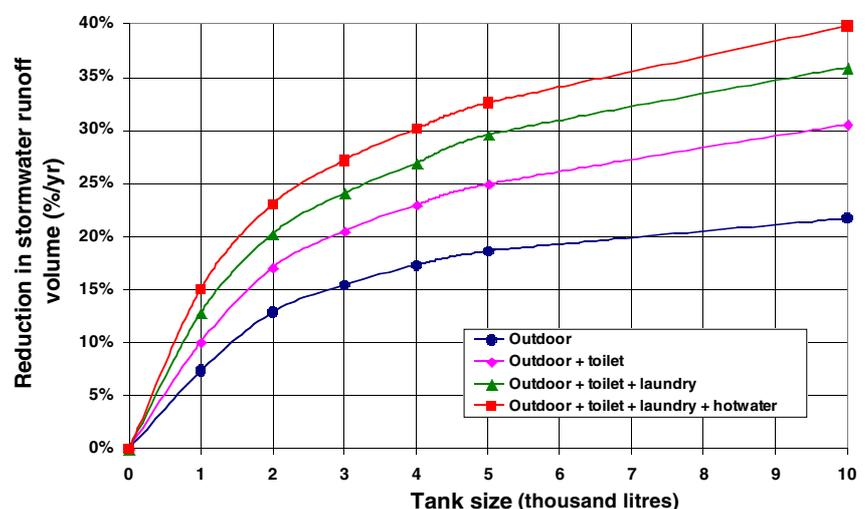
Fig 11: Reductions in annual stormwater runoff volumes provided by rainwater tanks at North Ryde for a 150 m<sup>2</sup> roof catchment
