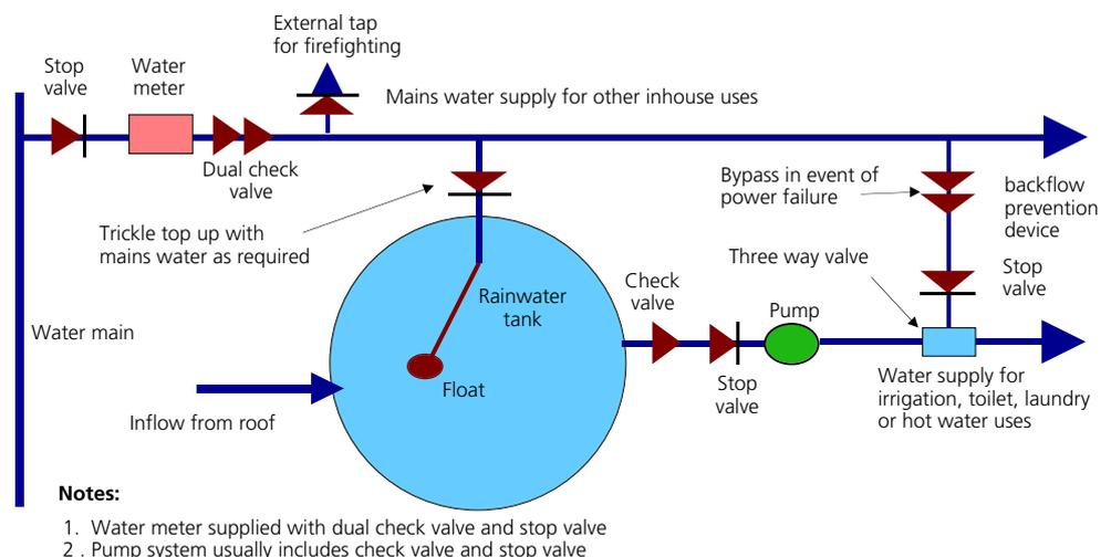
Fig 5: Configuration for a dual supply system with mains water trickle top up
