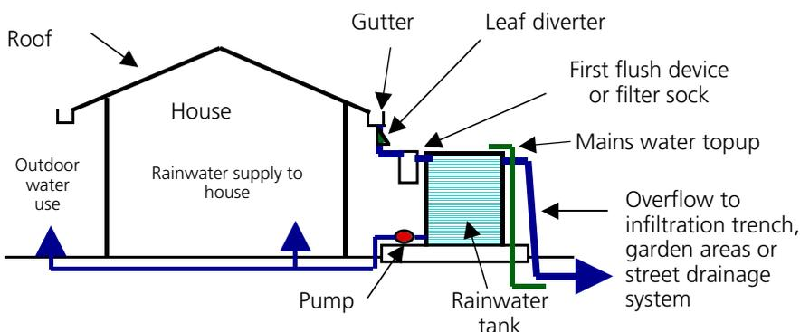
Fig 3: Elements of a domestic rainwater system (the rainwater treatment train)
